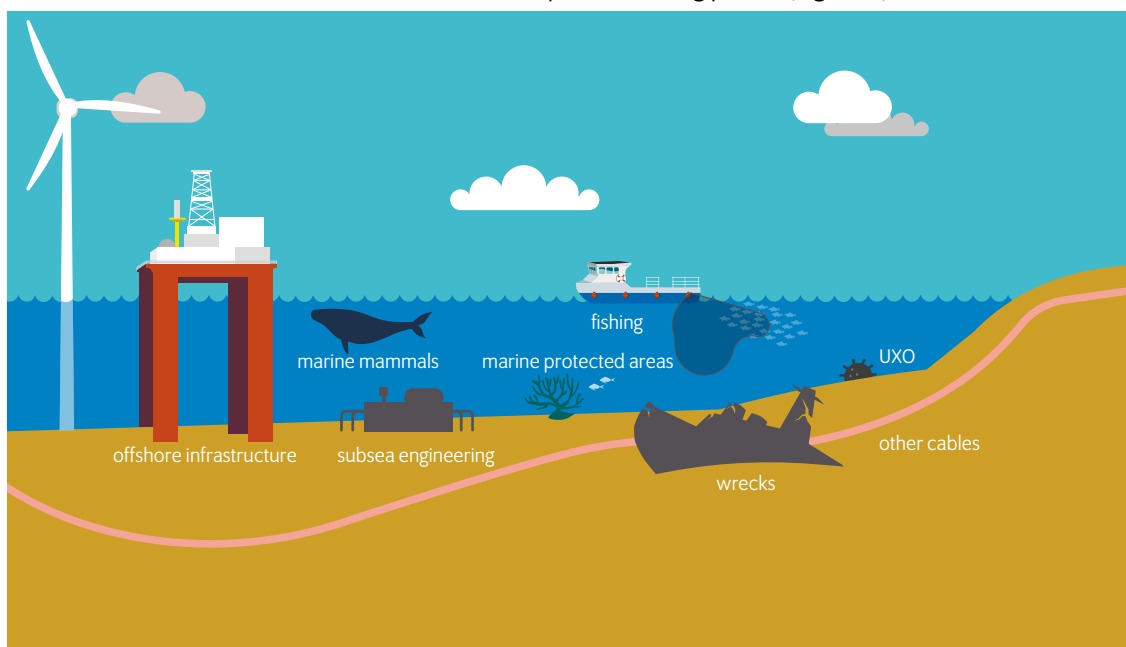
Figure 4 Potential cable interactions
