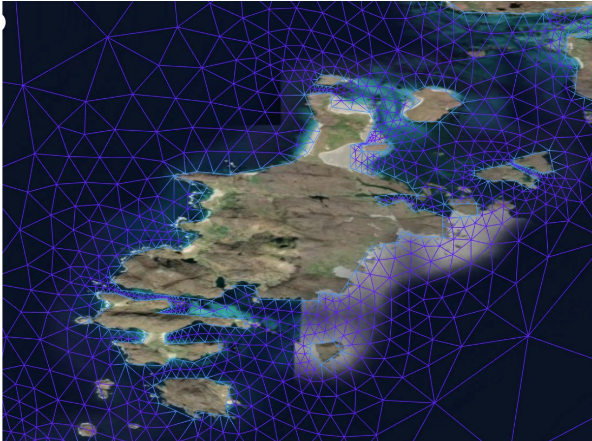
Figure 9 | Modelling domain for the Hebrides, showing boundaries and finite element mesh, close-up on Barra
